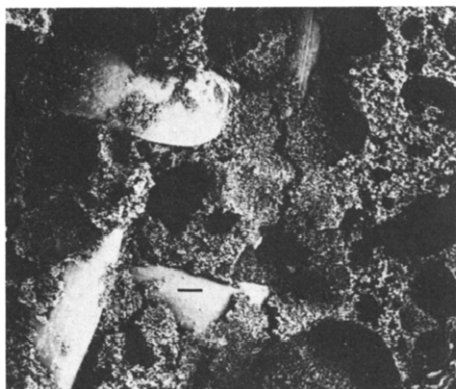
Fig 5 The coarse structure of the Zn(AQ) electrode, lying within the grid of the copper gauze (bar = 100 \mu\text{m} )
