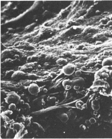
Fig 13 An edge view of the surface of the PVA20 electrode
